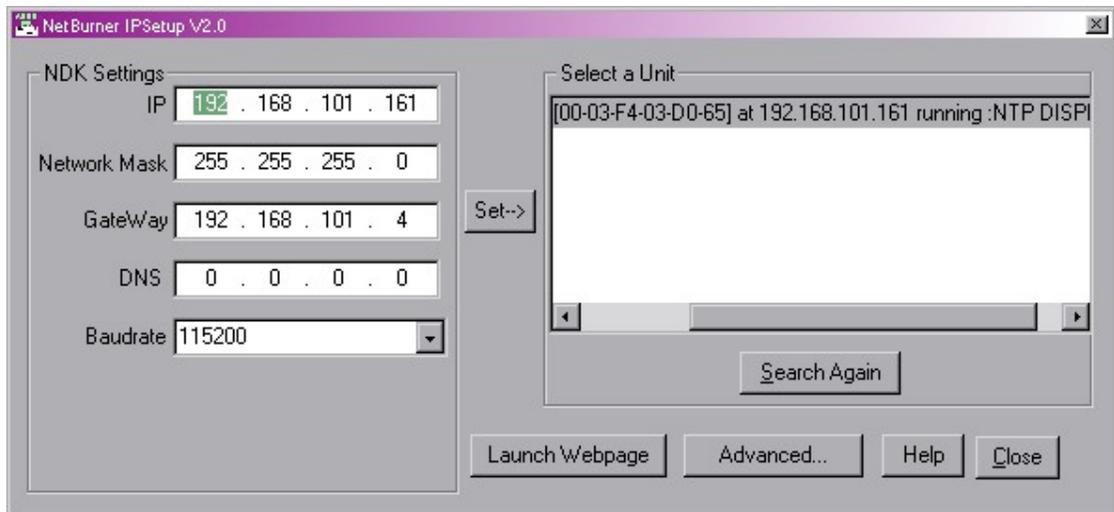
Select the required unit and alter the IP settings in the left hand pane to the required parameters (DNS and Baudrate are not needed). Click Set when complete and the unit is reset with these parameters. Once the unit's IP address is on the same subnet as the PC click 'Launch Webpage' to go to the unit.
